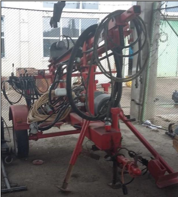
A water well trailer rig for shallow drilling.
